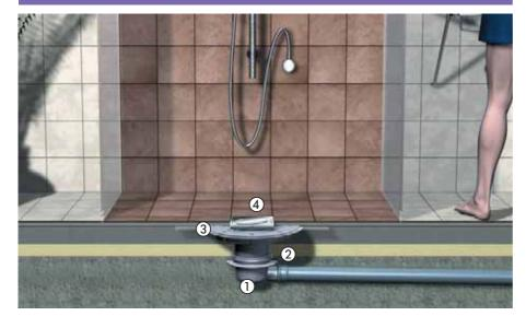
The *Classic* bathroom drain ① is a compact bathroom drain which is available in many versions. It is available both with a vertical and a horizontal outlet ② in the sizes  $\varnothing$  50 and  $\varnothing$  75 mm. There is an adhesive flange ③ available as an option for humidity sealing. The cover is a stainless steel cover in an oval design ④ - but *Classic* bathroom drain can also be combined with any other upper section from the System 100 range.
